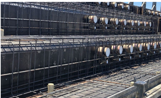
Figure 38: Bent WWR installed in forms for the production of precast concrete stadium risers.
