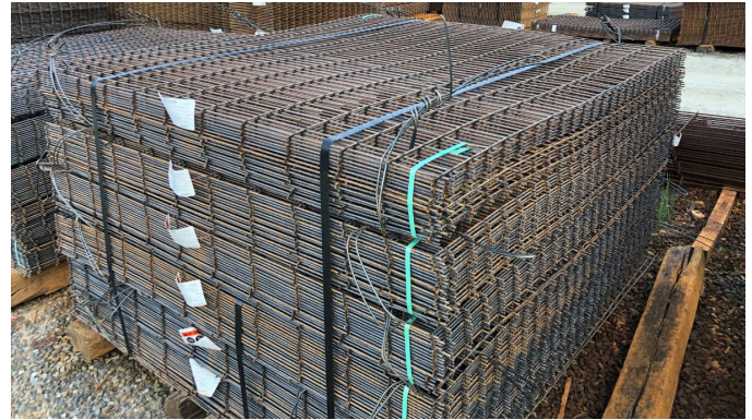
Figure 4: WWR bundles staged at the manufacturer's yard, with tags attached.
