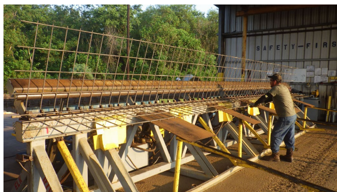
Figure 32: A long WWR mat on a bender. Note the alignment of wires with the individual bending mandrels, and the mat itself being pushed through an angle by the continuous rail arm behind.
