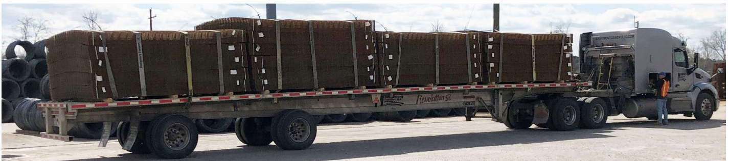
Figure 48: A truck loaded with a variety of WWR mats ready for transport to the site
