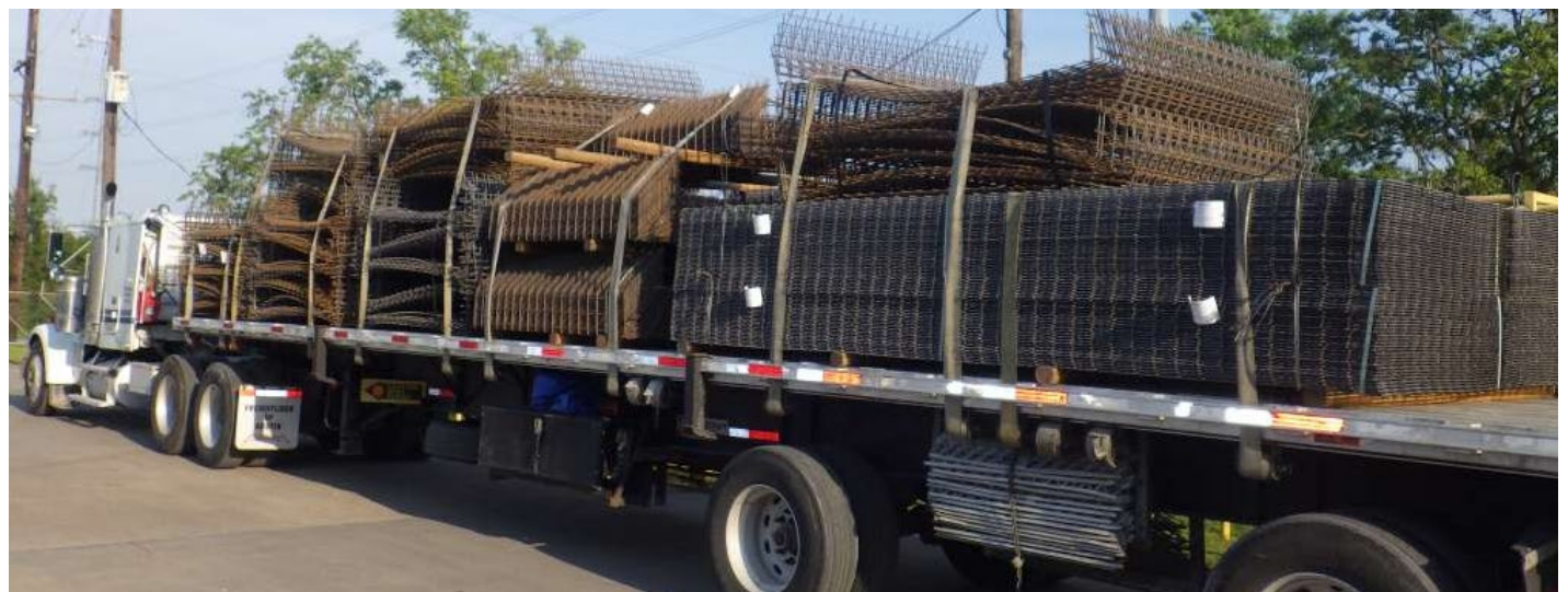
Figure 51: A combination of flat and bent WWR loaded on a truck, ready for transport. Placement of the various WWR mat bundles is carefully planned to maximize the amount of material that can fit on the truck without incurring violations related to dimensional and/or weight restriction.
