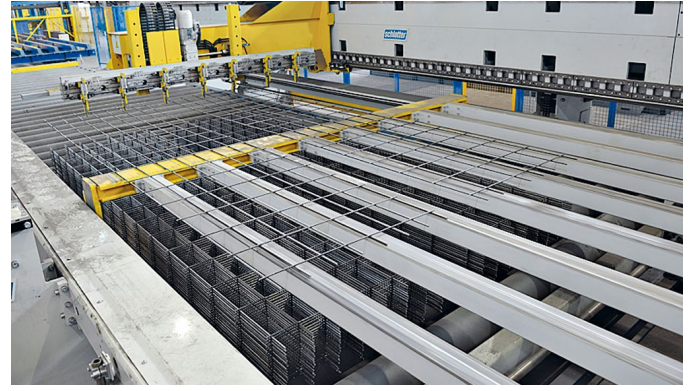
Figure 31: A view of the output side of the production line, showing completed WWR mats downstream of the welding station. Modern equipment is utilized to stack (as well as “flip” for better nesting of material within a bundle) the finished WWR mats. The WWR mats are then either transferred to a bending fabrication station or, for material to remain flat, directly to a staging area for subsequent loading onto trucks for delivery.
