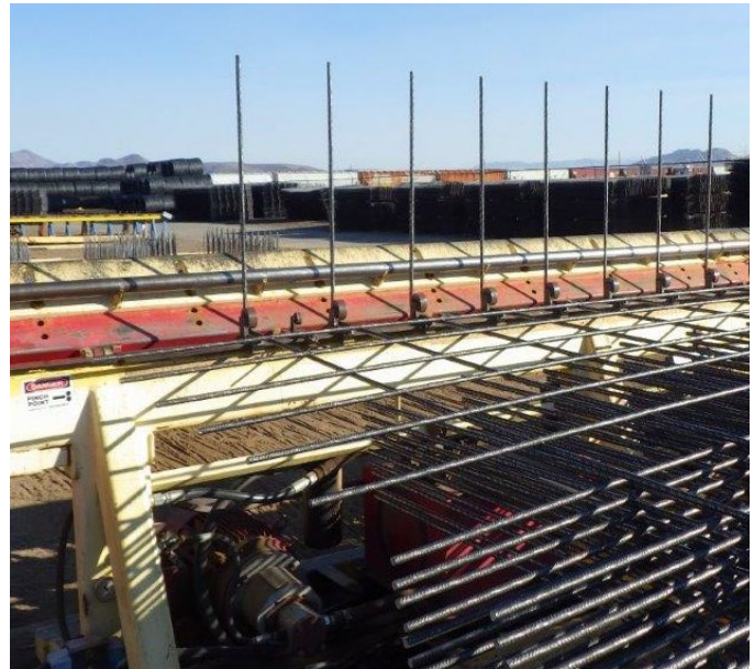
Figure 35: A WWR mat on a bender. Notice the staging of the remaining WWR mats to be bent as part of the scheduled bending operation.
