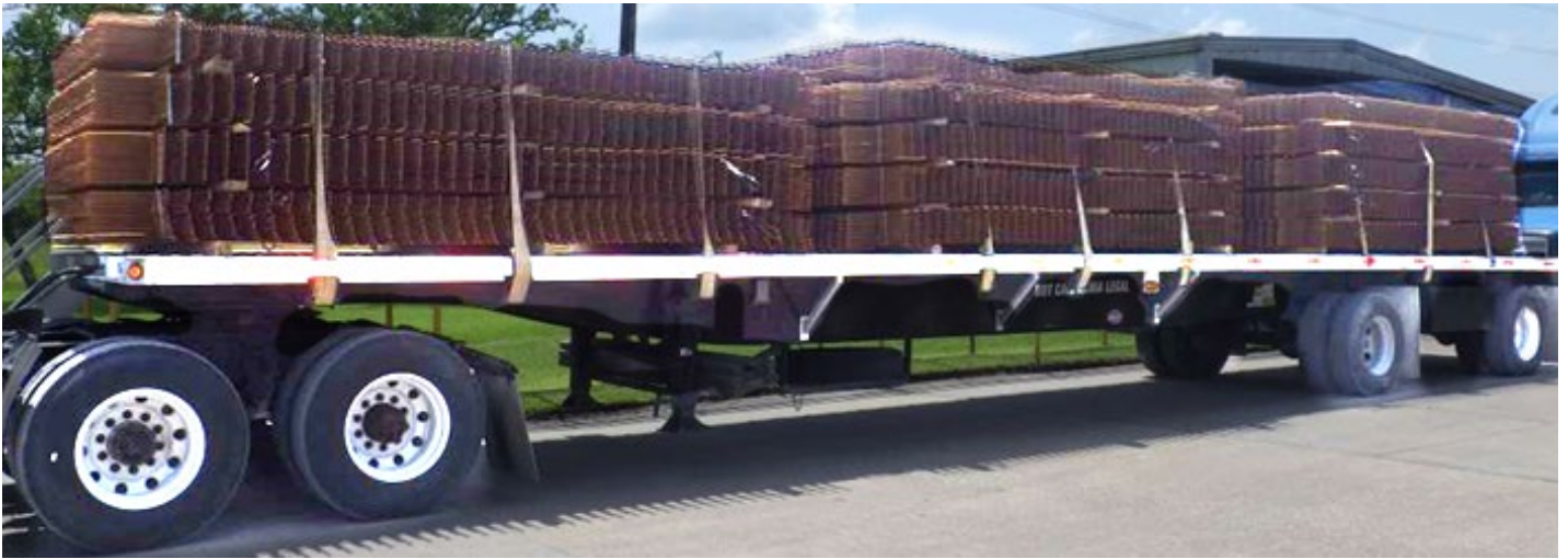
Figure 49: A truck loaded with a variety of WWR mats ready for transport to the site
