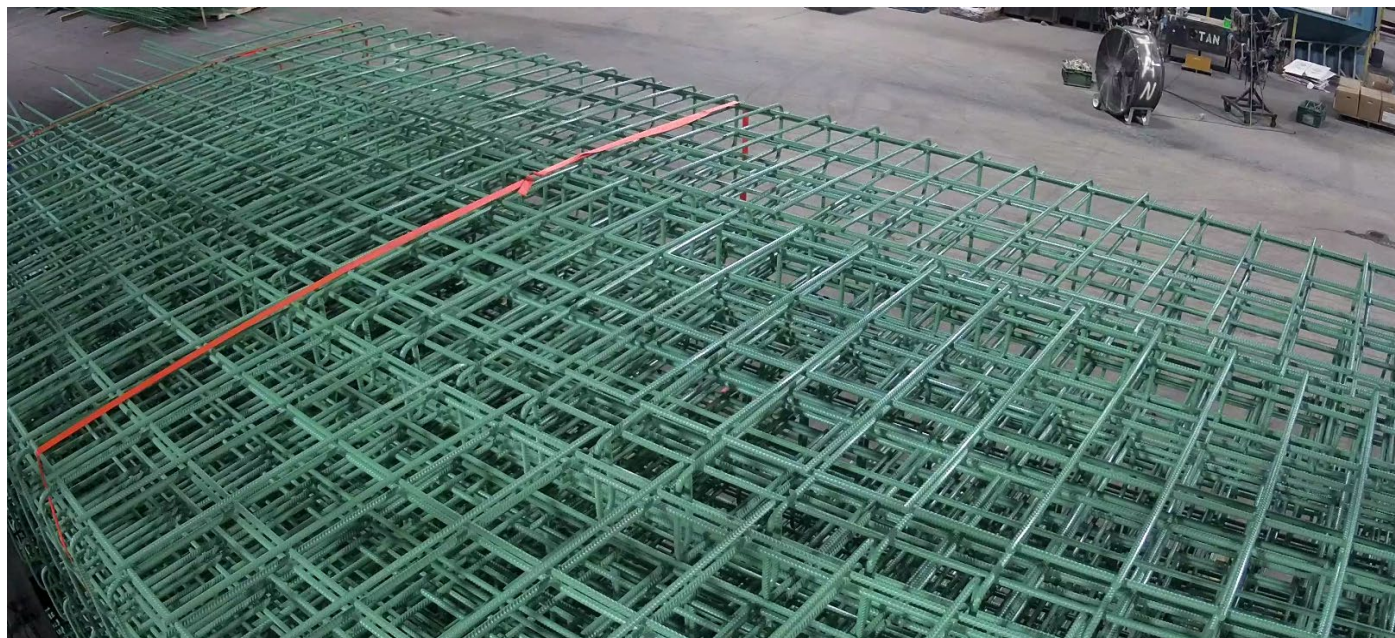
Figure 46: Bundled epoxy-coated WWR
