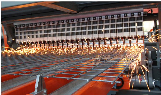
Figure 28: View of the welding electrode line in action.
