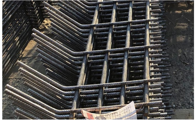
Figure 12: WWR mat bundle showing configuration to be used in a precast concrete application. Note the manufacturer-bent wire terminations.
