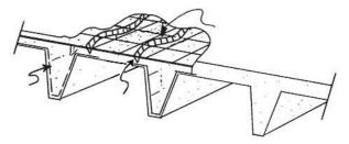
The maximum spacings and minimum steel areas (see ACI 318, Section 24.4) in Table I are for wires in both directions.
