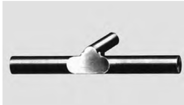
Figure 1.1. Section at typical weld showing complete fusion of intersecting wires.
