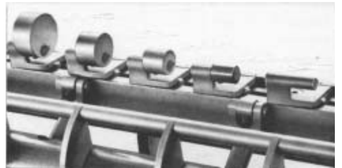
Various mandrel sleeve diameters can be used to obtain desired bending radii.
