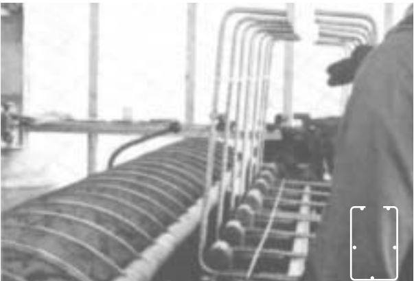
COMPLETION: Stirrup is completed and ready for removal from the machine.
