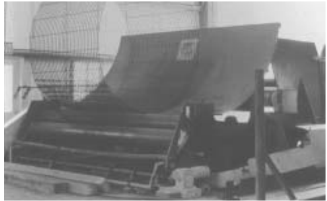
Welded Wire Reinforcement manufactured for concrete pipe.
