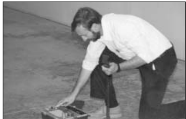
Professor Snell and the battery-powered cover meter used to detect placement of WWR reinforcement in the industrial slabs.
