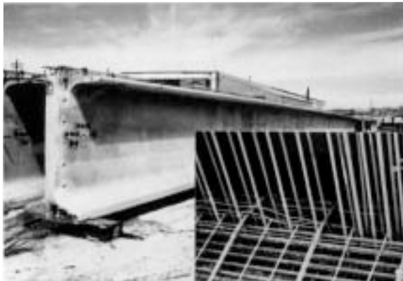
A 150-ft. bridge "I" girder shown being developed by Dr. Maher Tadros and his students at the University of Nebraska in 1992. This prestressed girder and others like it and some with even longer spans are being designed into bridges in many states across the country.
